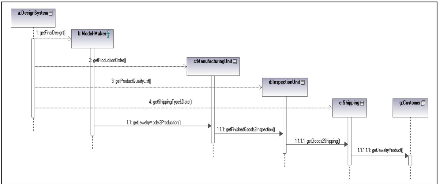
Figure 4: The UML Sequence Diagram of Design System–Associating (Inside Enterprise) Facility Interactions.
