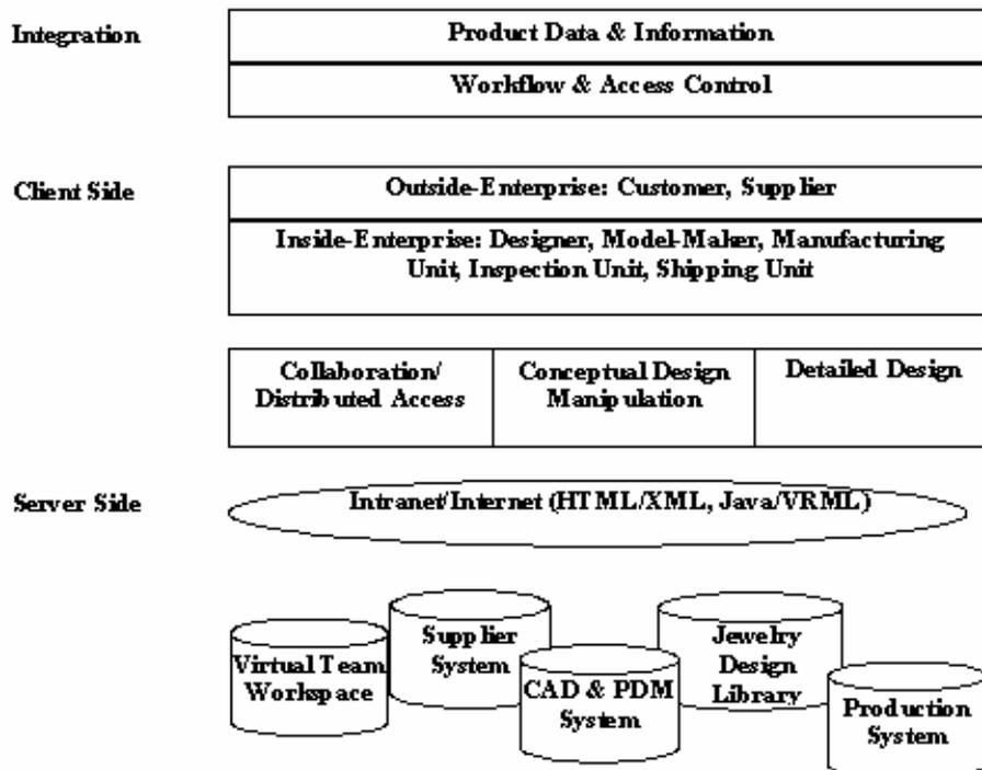
Figure 2: System architecture of collaborative design & manufacturing system.
